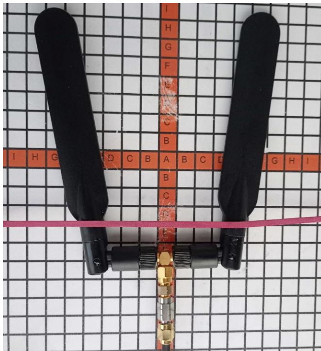
2D field scan - a pair of WiFi antennas (2.4 GHz, case 3)
